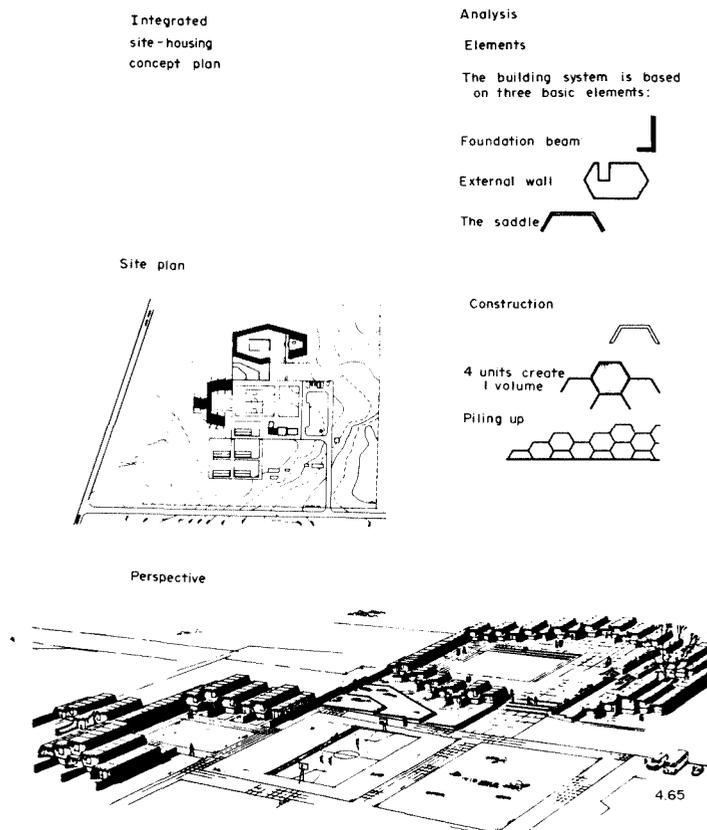
Fig. 13. Integrated Site-Housing Plan.
