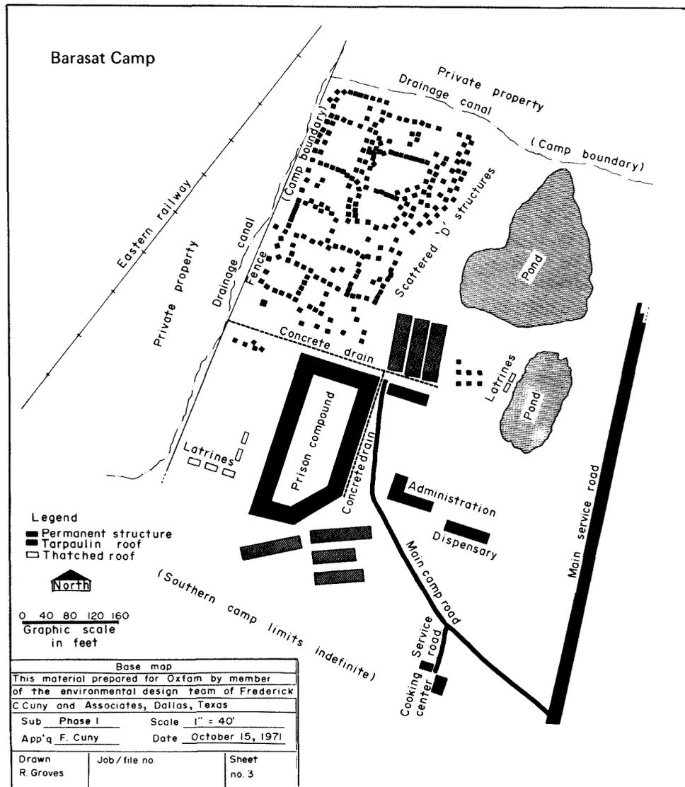
Fig. 1. Barasat Camp (W. Bengal, India 1971): This drawing illustrates a typical Phase I camp. It was built on government lands surrounding a prison. Note the shelters which were constructed on the embankments of rice paddies and have no scheme of layout.
